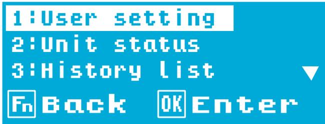
From the function menu, you can navigate with the UP and DOWN button, return to previous page with the BACK button, and enter the selected item with the OK button.
