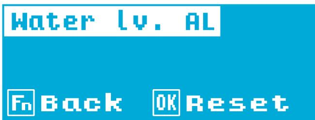
After the conditions which caused the fault have been corrected, you can reset the alarm by pressing the OK button. The interface will then return to the main display and the unit operate normally.
